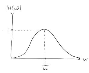
$$H(\omega) = \frac{R}{R + 3\omega L} + \frac{1}{3\omega C} = \frac{3\omega RC}{1 - \omega^2 LC + j\omega CR}$$
