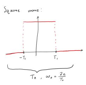
$$C_{o} = \frac{2T_{i}}{T_{o}} \qquad C_{k} = \frac{2}{T_{o}k\omega_{o}} \sin(k\omega_{o}T_{i})$$
