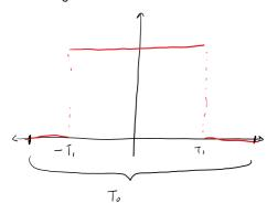
$$C_{o} = \frac{1}{T_{o}} \int f(t) \, \partial t = \frac{1}{T_{o}} \cdot 2T_{i} = \frac{2T_{i}}{T_{o}}$$
