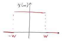
fourier transform  $\chi(j_w)$ :  $\chi(t) = \frac{1}{2\pi} \int_{-\infty}^{\infty} \chi(j_w) e^{jwt} dt = \frac{1}{2\pi} \int_{-\infty}^{\infty} e^{jwt} dw$  $= \frac{1}{2\pi} \left[ \frac{e^{j\omega t}}{jt} \right]^{w} = \frac{1}{2\pi} \left[ \frac{e^{j\omega t} - e^{-j\omega t}}{jt} \right]$
